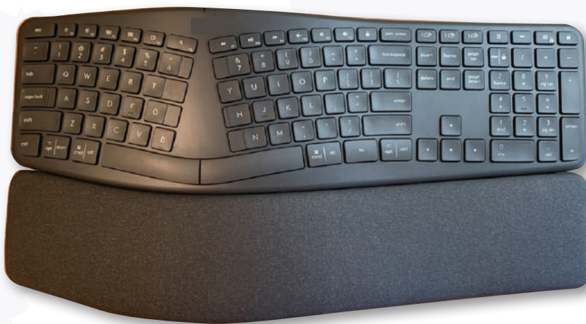
Figure 7.9 : Example of ergonomics keyboard well-for sparing arms and wrists when typing
